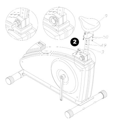
**2.** Attach the seat (9) to the seat post (3) with the locknuts (49) and flat washers (50) already provided on the underside seat bolts.
